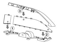
3. Insert the three knobs on the cable cover into the three holes on the projector as shown in the figure. Pass the cables through the holes on the bottom of the cable cover.
